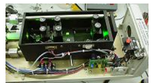
Close-up of the SHG cavity. Six adjustment knobs are provided for fine-tuning the output.
